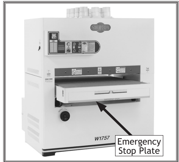
Figure 19. Emergency stop plate.
